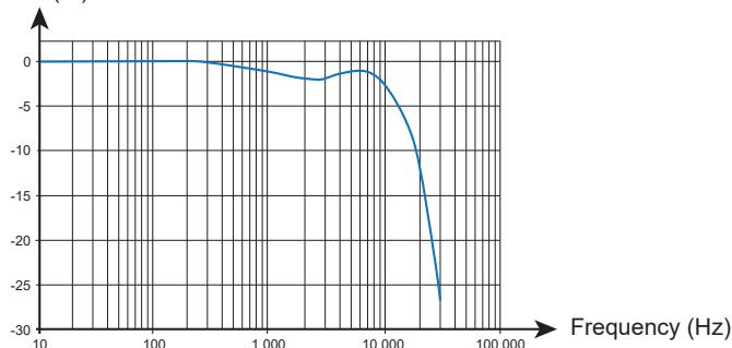
Typical phase error versus frequency curve at 100A
