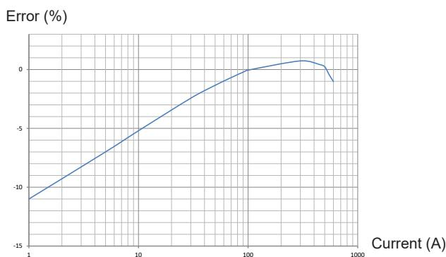
Typical phase error curve at 60Hz
